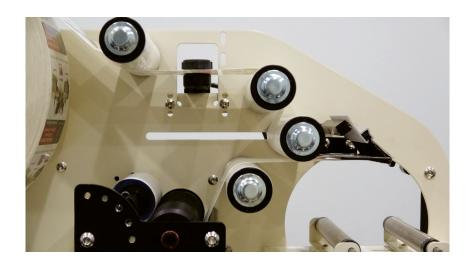
3. Slide the label stop roller (28C) toward the back of the machine in small amounts. As the roller is moved back, the stop position of the label will be adjusted. Continue moving roller until a label gap is stopping at the Peel Plate (1).
