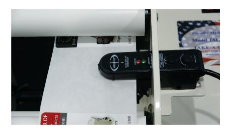
**3.** Press and hold the "Normal" button on photo eye for 3 seconds. When the lights finish flashing the photo eye is taught.
